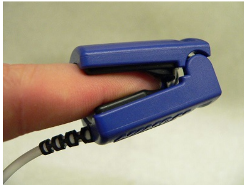
Figure 1: A fingertip pulse oximeter uses PPG to measure heart rate.
